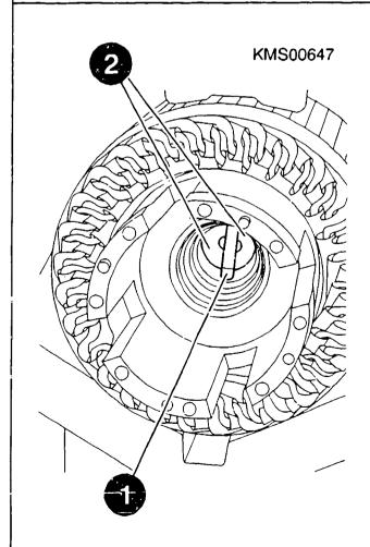
Replacing needle bearing in armature Installing:
